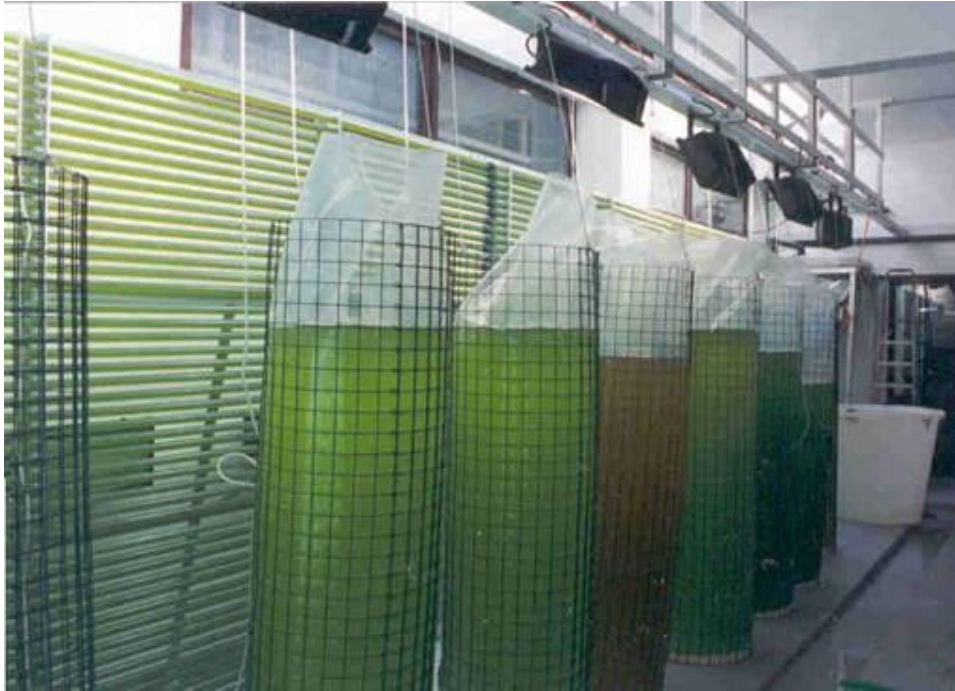
Biofence system and conventional bags for cultivation of microalgae in a hatchery in Greece.
